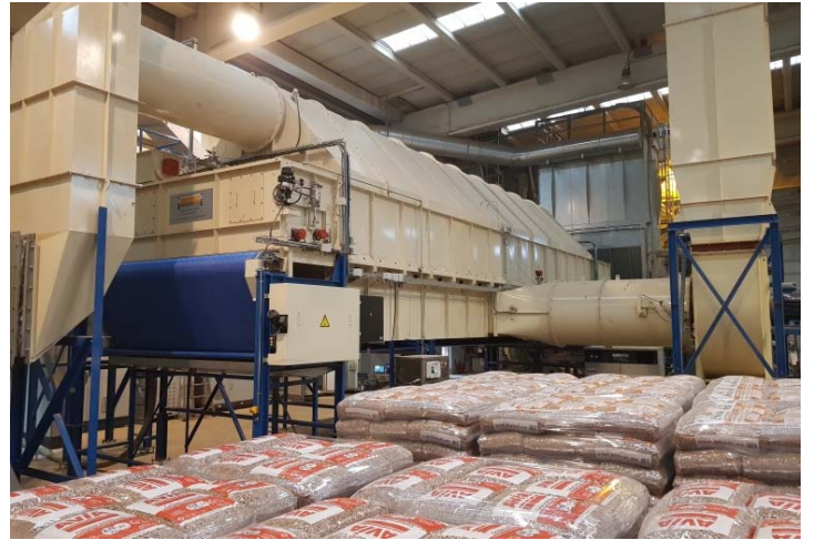
Low temperature belt dryer
